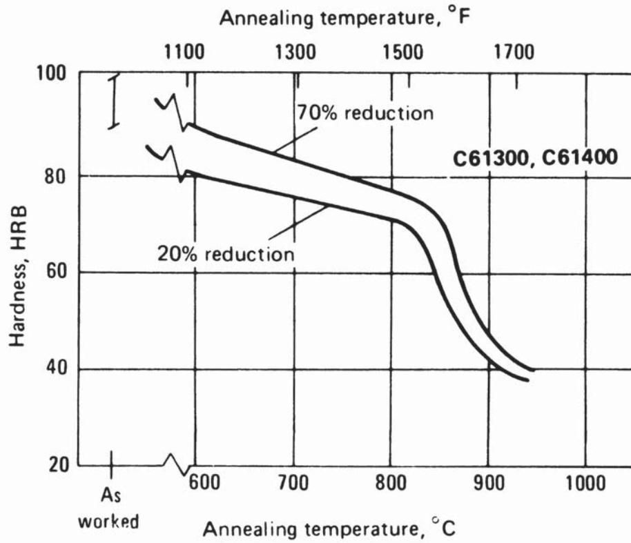
Annealing curves for cold-reduced alpha-aluminum bronzes. Time at annealing temperature, 1 h. Source: *ASM Handbook, Vol. 4, Heat Treating*, ASM International, 1991, p 897
