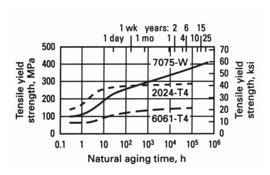
Natural aging curves for three solution heat-treated wrought aluminum alloys. Source: J.R. Davis, Ed., *Aluminum and Aluminum Alloys, ASM Specialty Handbook*, ASM International, 1993, p 35
