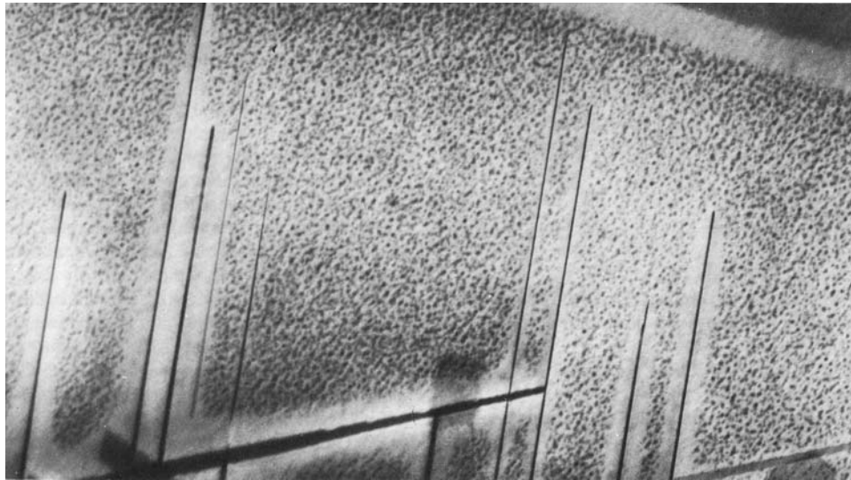
GP zones (dark spots) in the matrix of an Al-15Ag alloy dissolving near plates of the more stable precipitates (dark lines). Transmission electron micrograph of a specimen aged 1,200 h at 160°C (320°F). 23,000 \times . Source: J.R. Davis, Ed., Aluminum and Aluminum Alloys , ASM Specialty Handbook , ASM International, 1993, p 291
