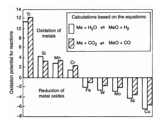
Oxidation potential of alloying elements and iron in steel heated in endothermic gas with an average composition of 40% H, 20% CO, 1.5% CH4, 0.5% CO2, and 0.28% H2O (Dew point, 10?C), and 37.72% N2. Source: *Carburizing: Microstructures and Properties*, by Geoffrey Parrish, ASM International, 1999, p 12
