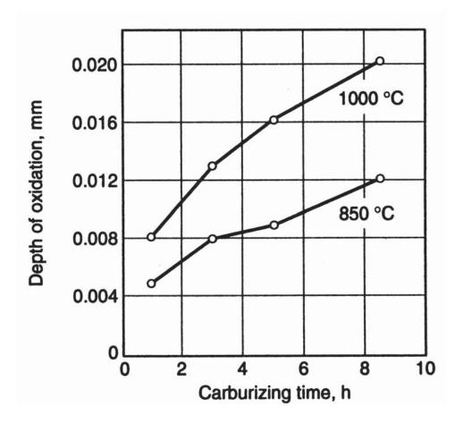
Depth of the oxidized zones versus carburizing time at different carburizing temperatures for SAE 1015. Source: *Carburizing: Microstructures and Properties*, by Geoffrey Parrish, ASM International, 1999, p 13
