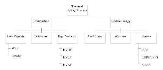
Figure 3a: Types of Thermal Spray Processes (HVOF: High Velocity Oxy-Fuel; HVLF: High Velocity Liquid-Fuel; HVAF: High Velocity Air-Fuel; APS: Air Plasma Spray; LPPS/LVPS: Low Pressure Plasma Spray/ Low Vacuum Plasma Spray; CAPS: Controlled Atmospheric Plasma Spray)
