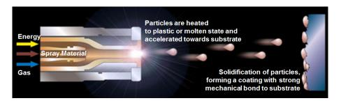
Figure 2b: Principle of Thermal Spray Coatings
