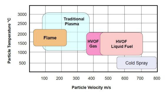
Figure 4a: Overview of Particle Temperature versus Particle Velocity for Different Processes
