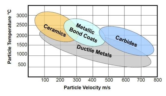
Figure 4b: Overview of particle temperature versus particle velocity for different materials systems
